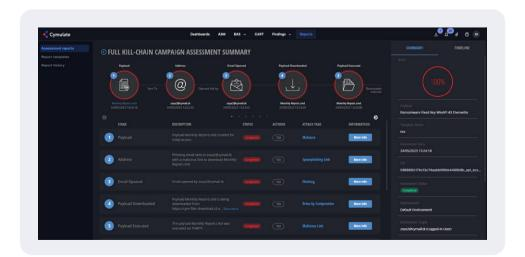
The full kill-chain campaign assessment summary provides a graphical representation of the attack stages at the top of the screen. Each stage in the attack that was executed successfully is circled in red, and the stage that is circled in orange is the stage the attack was thwarted. The full kill-chain stages are also listed below, each row displaying the stage, its description, status, actions, and ATT&CK tags.
