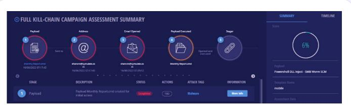
The full kill-chain campaign assessment summary visually represents the attack stages at the top of the screen. Each stage in the attack that was executed successfully is circled in red, and the stage that is circled in orange is when the attack was thwarted. The full kill-chain stages are listed below, each row displaying the stage, its description, status, actions and ATT&CK tags.
